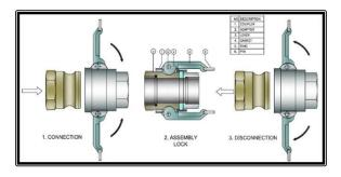
Rated Working Pressure @ 20°C : 15mm - 50mm 150psi, 65mm 125psi, 100mm 100psi & 150mm 75psi,
