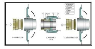
Rated working pressures at 20° C 15mm – 25mm 100psi, 40mm – 50mm 75psi, 80mm – 100mm 50psi As a guide only, polypropylene may be suitable for -9°C to +90°C (WATER) but rated working pressures drop significantly with polypropylene camlocks. Special precaution must be taken when using at elevated temperatures - consult factory.
