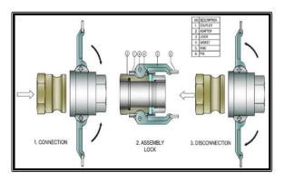
Rated working pressures at 20° C 15mm – 25mm 100psi, 40mm – 50mm 75psi, 80mm – 100mm 50psi Maximum temperature is 79°C. Special precaution must be taken when using at elevated temperatures - consult factory.
